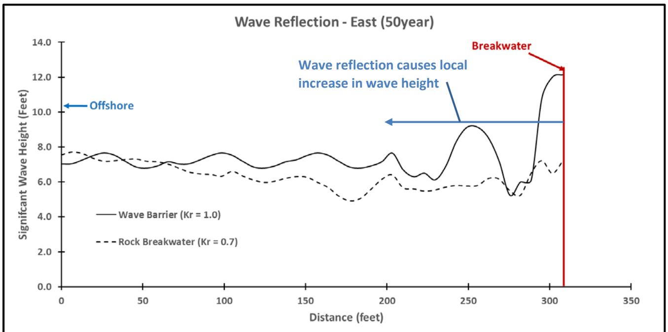
Figure 16. Wave Height Comparison near Tip of Wave Barrier and Rock Breakwater – Waves from East (50-year Return Period)
