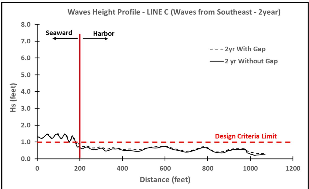
Figure 20. Wave Height Comparison – LINE C - Waves from the Southeast (2-year)
