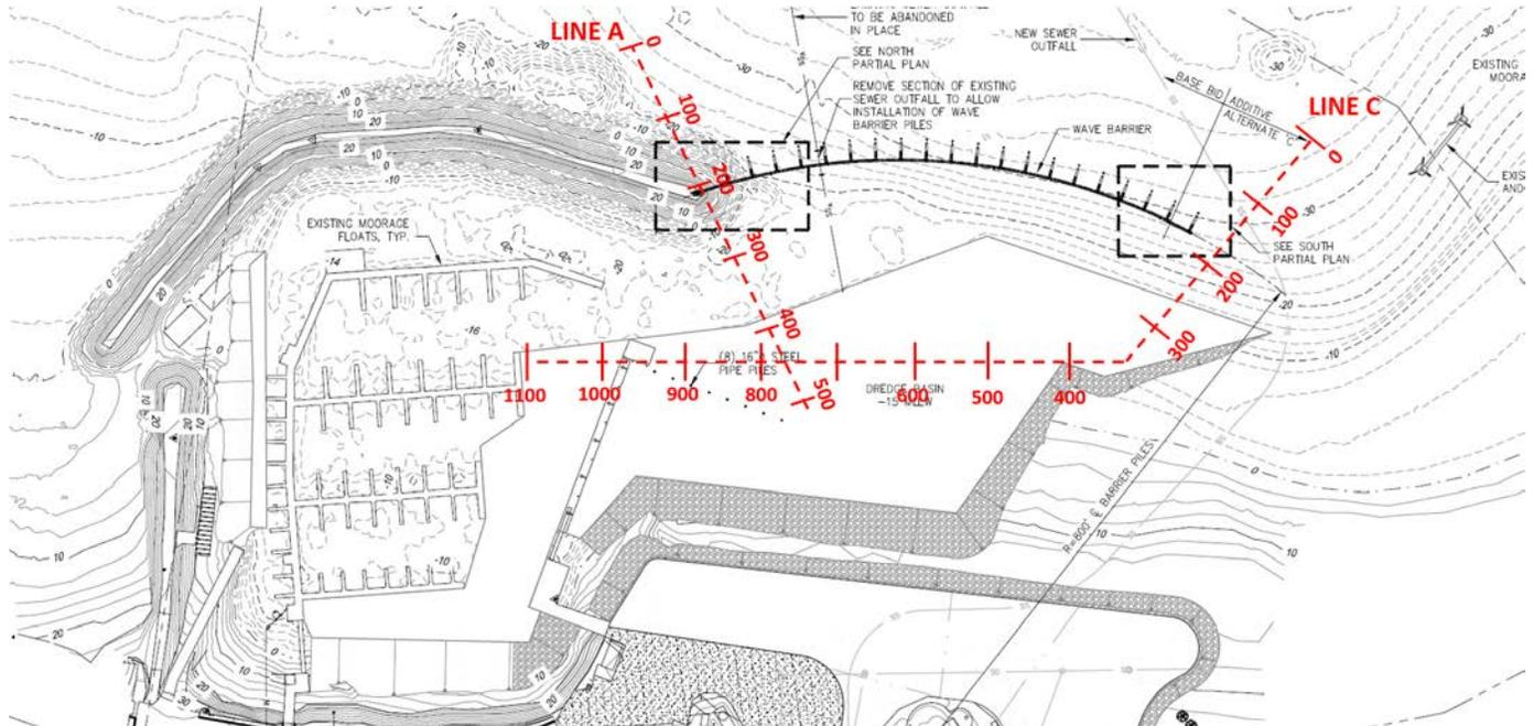
**Figure 6. Wave Height Output Locations**
