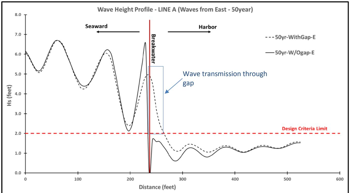
Figure 8. Wave Height Comparison – LINE A - Waves from East – 50 year Return Period ( $H_s = 6.6$  ft,  $T_p = 4.5$ s)
