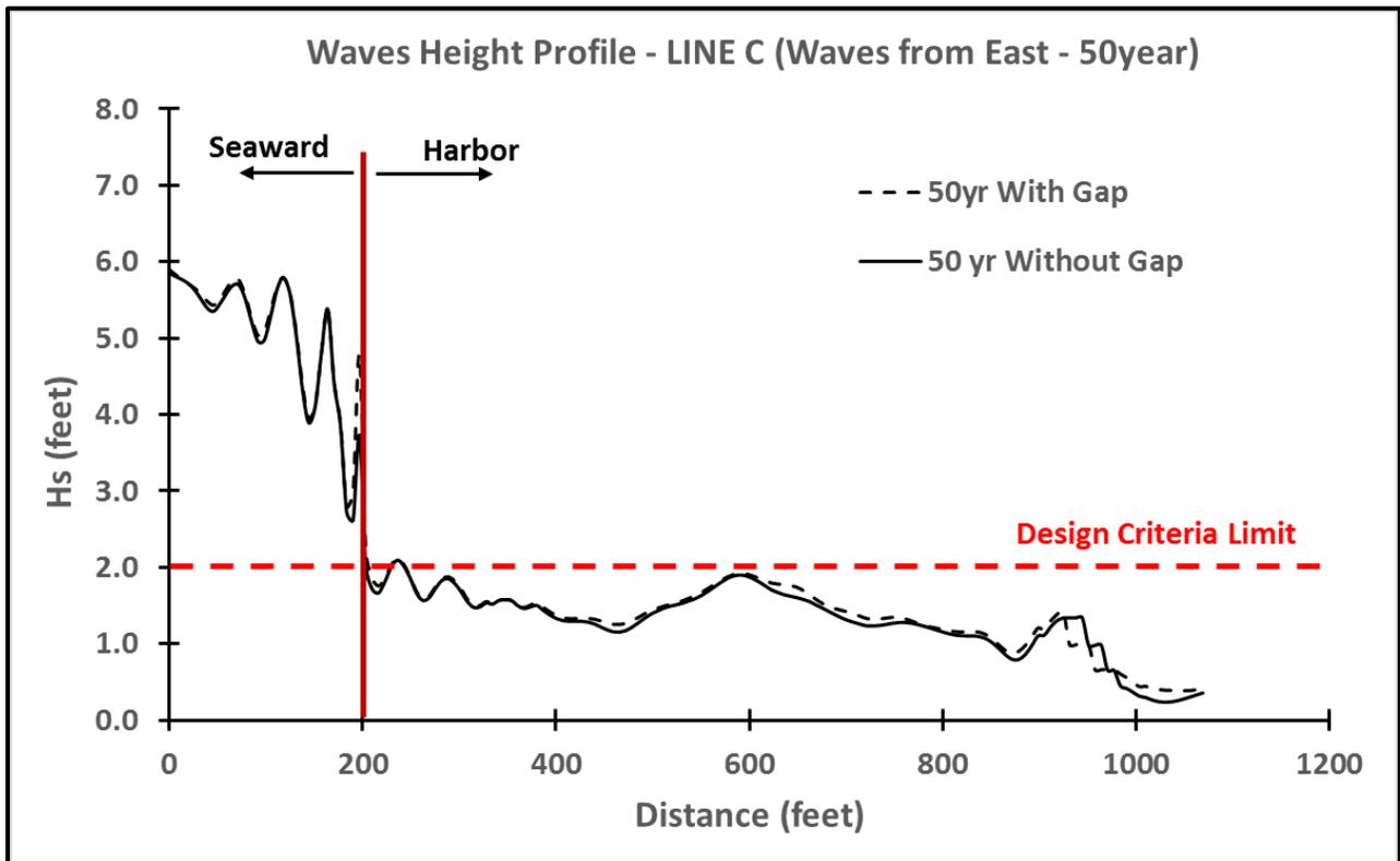
Figure 19. Wave Height Comparison – LINE C - Waves from the East (50-year)
