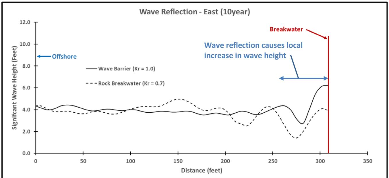
Figure 15. Wave Height Comparison near Tip of Wave Barrier and Rock Breakwater – Waves from East (5-year Return Period)
