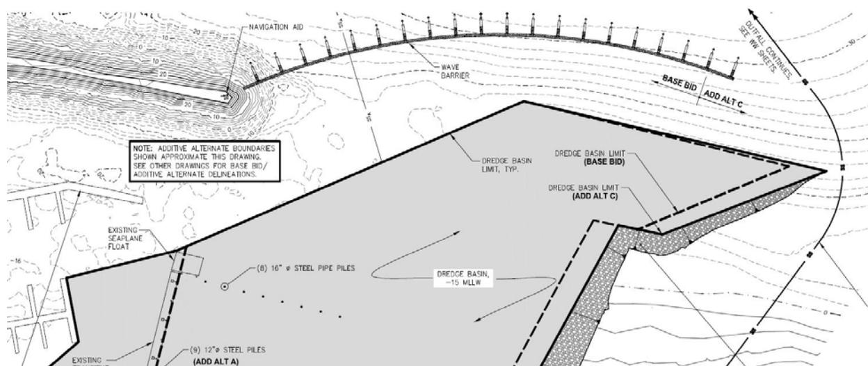
**Figure 1. Alternative 1 - PCHE Wave Barrier – 95% Design with Gap (Length 633 feet)**
