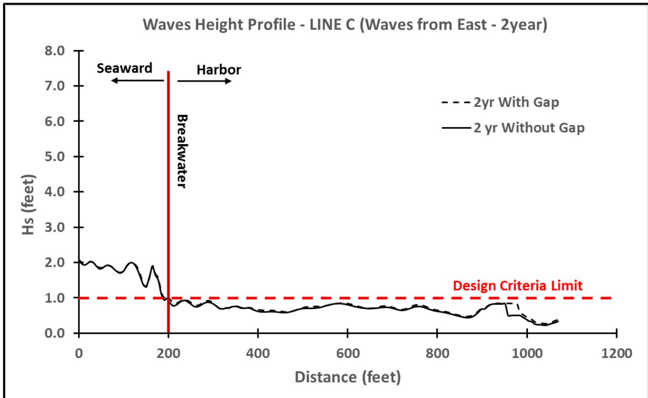
**Figure 18. Wave Height Comparison – LINE C - Waves from the East (2-year)**
