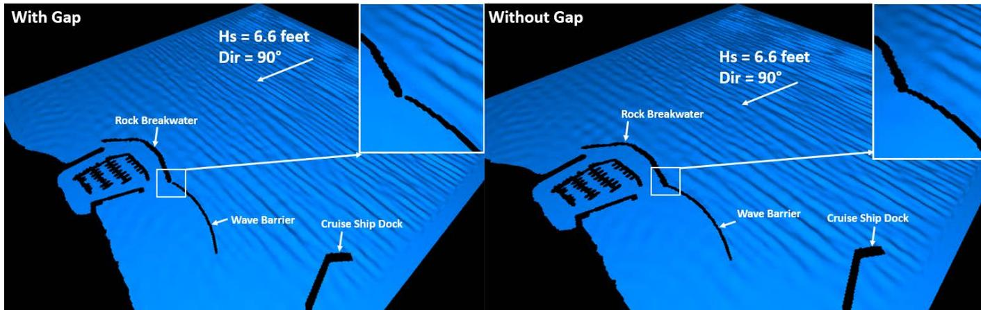
Figure 11. Model Animation Screenshots – Water Surface for Waves from east (Azimuth 090°)
