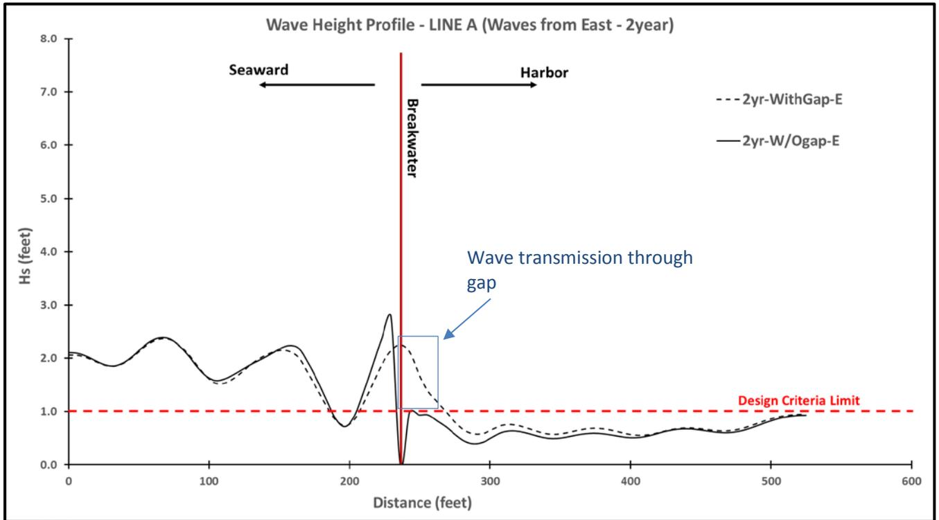
Figure 7. Wave Height Comparison – LINE A - Waves from East – 2 year Return Period ( $H_s = 2.6$  ft,  $T_p = 4.5$ s)
