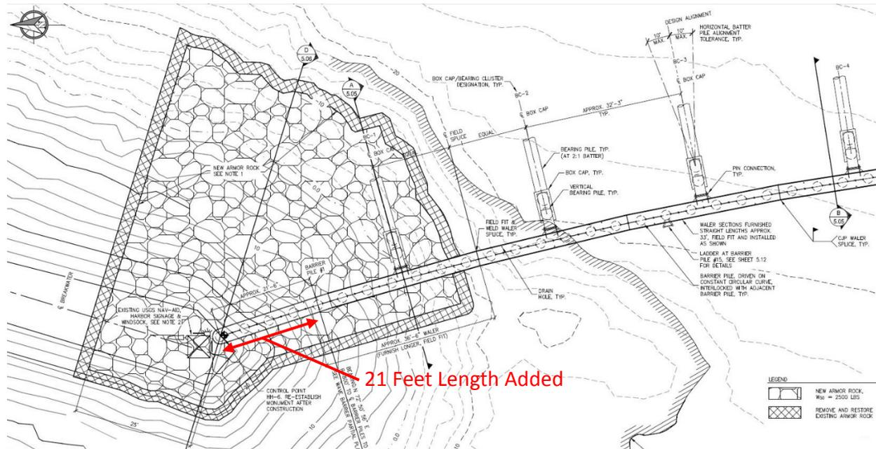
Figure 2. Alternative 2 Partial Plan - PCHE Wave Barrier without Gap (Length 654 feet)
