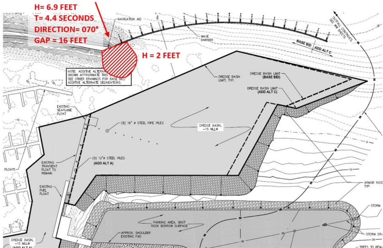
Figure 4. Wave Transmission at Gap - Diffraction Diagram Analysis – 50 Year Return Period Wave
