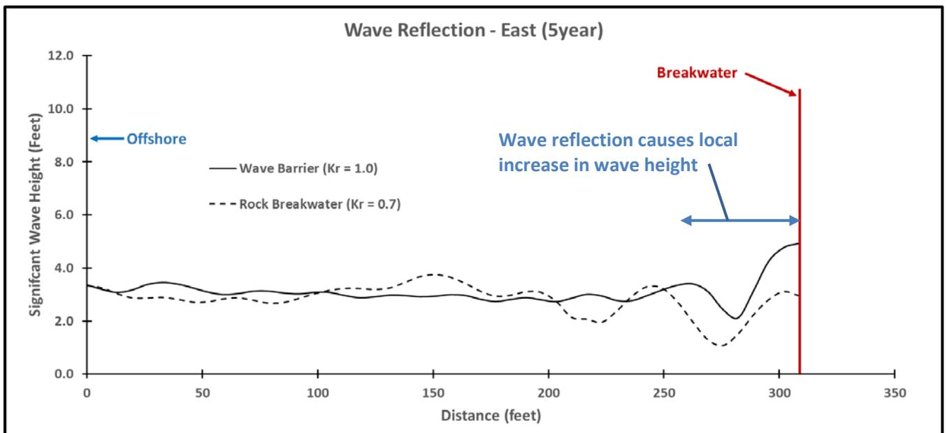
Figure 14. Wave Height Comparison near Tip of Wave Barrier and Rock Breakwater – Waves from East (5-year Return Period)
