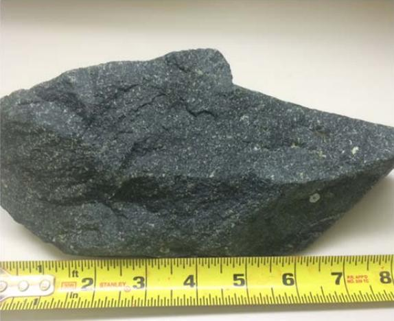
Fragment of armor rock retained for laboratory testing
