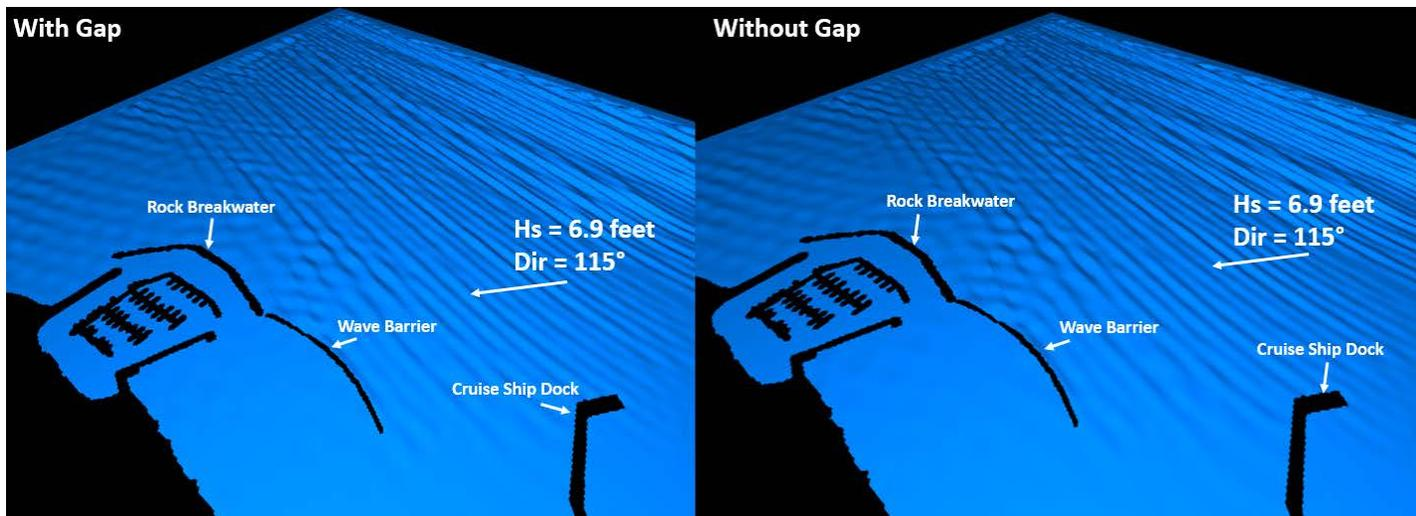
Figure 22. Model Animation Screenshots – Water Surface for Waves from southeast (Azimuth 115°)
