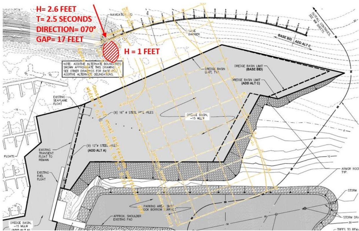
Figure 3. Wave Transmission at Gap - Diffraction Diagram Analysis – 2 Year Return Period Wave
