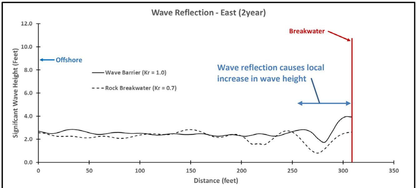
Figure 13. Wave Height Comparison near Tip of Wave Barrier and Rock Breakwater – Waves from East (2-year Return Period)
