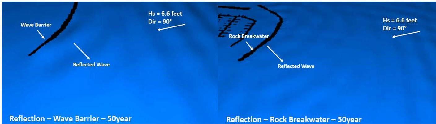
**Figure 17. Animation Screenshot - Wave Height Comparison near Tip of Wave Barrier and Rock Breakwater – Waves from East (50-year Return Period)**
