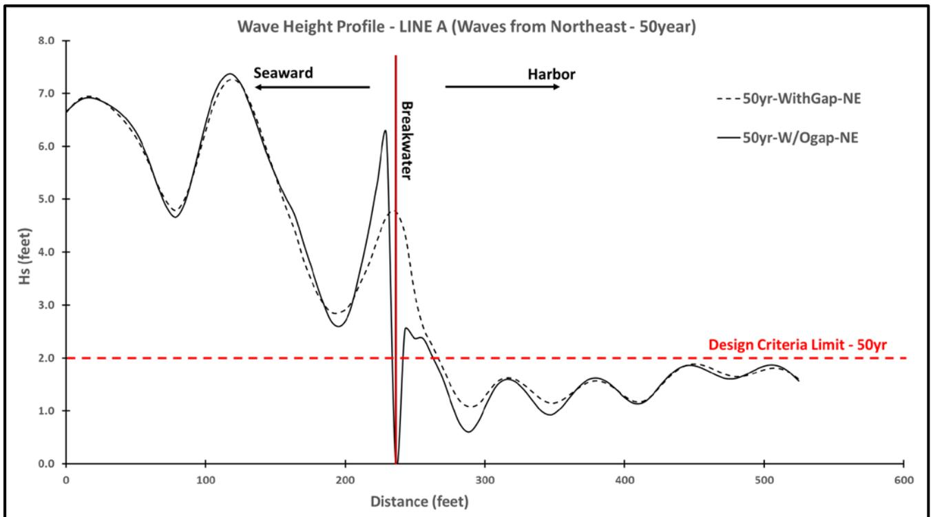
Figure 10. Wave Height Comparison – LINE A - Waves from Northeast – 50 year Return Period ( $H_s = 6.5$  feet,  $T_p = 4.5$  seconds)
