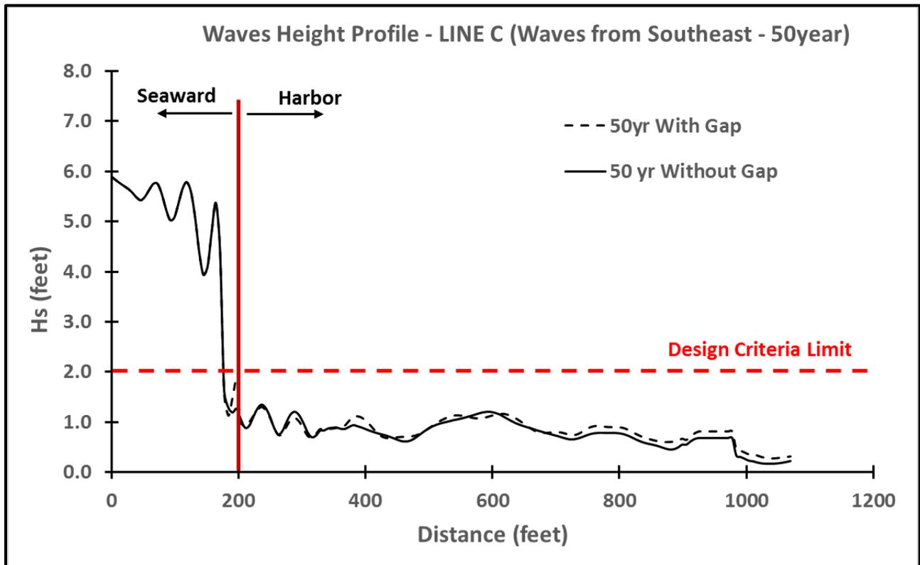
Figure 21. Wave Height Comparison – LINE C - Waves from the Southeast (50-year)
