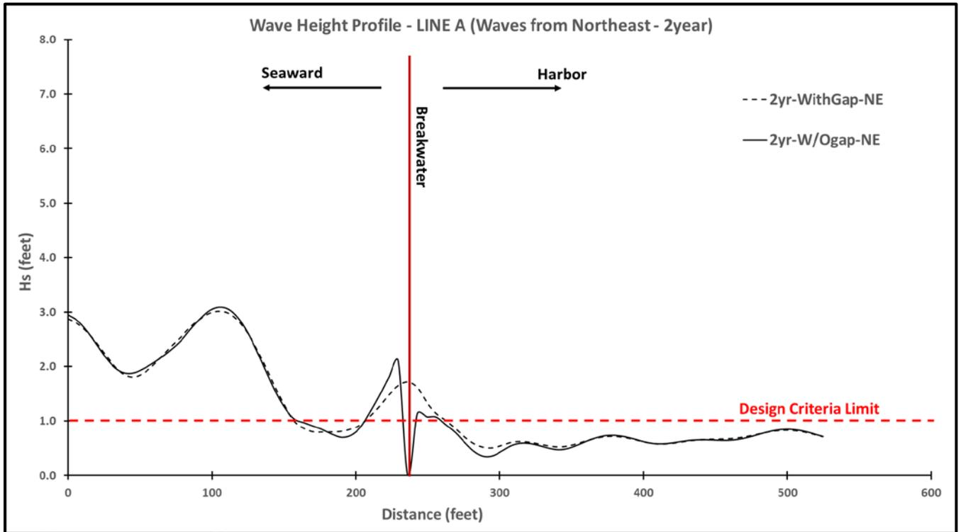
Figure 9. Wave Height Comparison – LINE A - Waves from Northeast – 2 year Return Period ( $H_s = 3.2$  ft,  $T_p = 4.5s$ )
