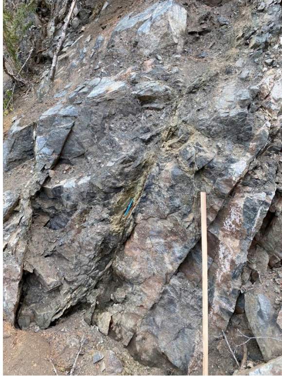
A: 10-inch wide shear/fault near parallel to layered rock at elev. ~830 ft in eastern lateral scarp.
