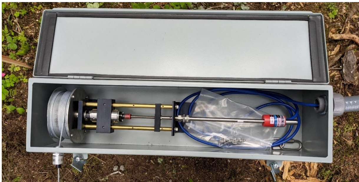
Photo 2: Long range displacement meter drum, lead screw, displacement transducer, and temperature sensor.
