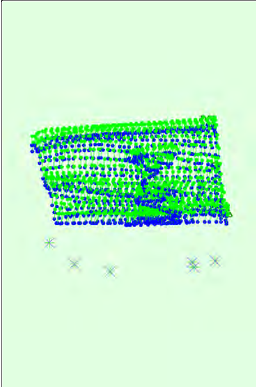
Figure 3: Offset between initial (blue dots) and computed (green dots) image positions as well as the offset between the GCPs initial positions (blue crosses) and their computed positions (green crosses) in the top-view (XY plane), front-view (XZ plane), and side-view (YZ plane). Dark green ellipses indicate the absolute position uncertainty of the bundle block adjustment result.
