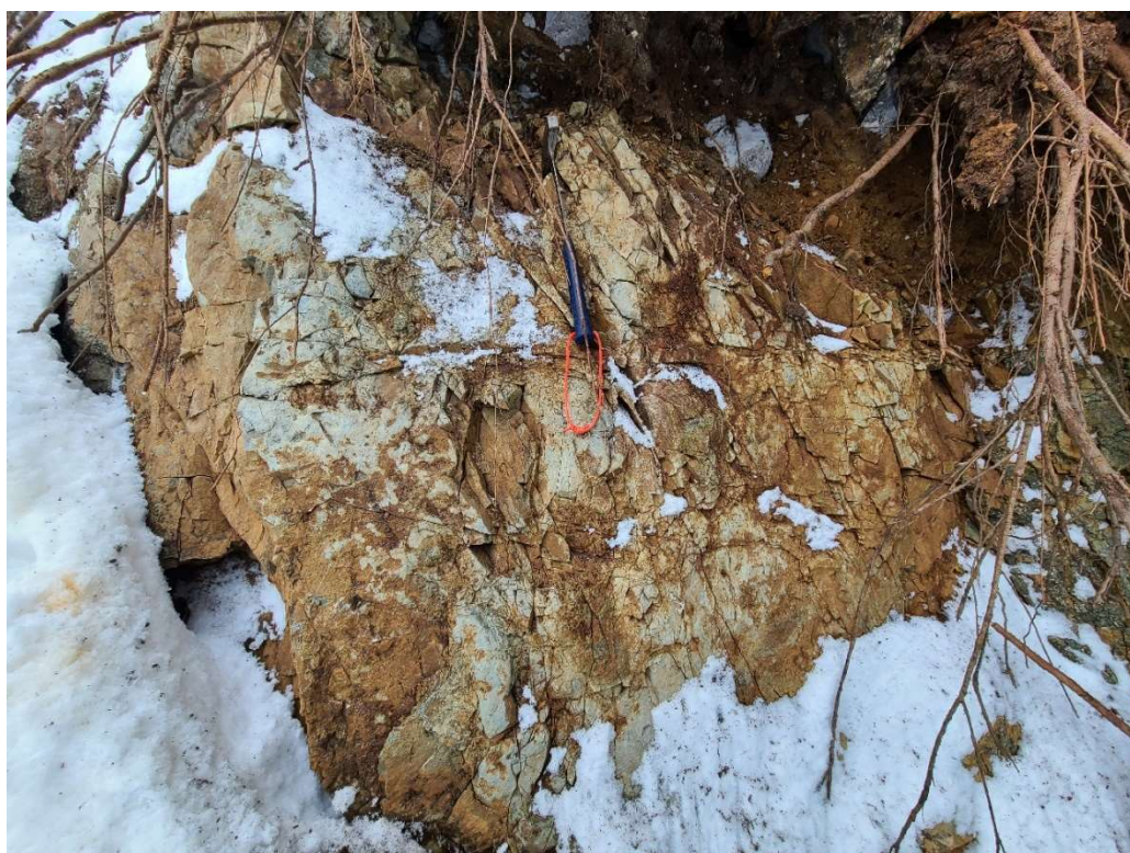
Close up view of the rock exposed in the western portion of the headscarp. Note altered nature of the rock surface (taken 2/23/2021).
