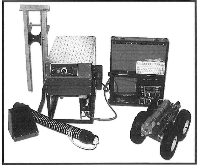
The USABlueBook Mainline Camera System w/Wheeled Transporter. Pictured with the PCU is the portable mainline reel, aluminum manhole roller, cable guide hose, transporter, zoom pan & tilt camera with plug-in remote, and viewing box.
