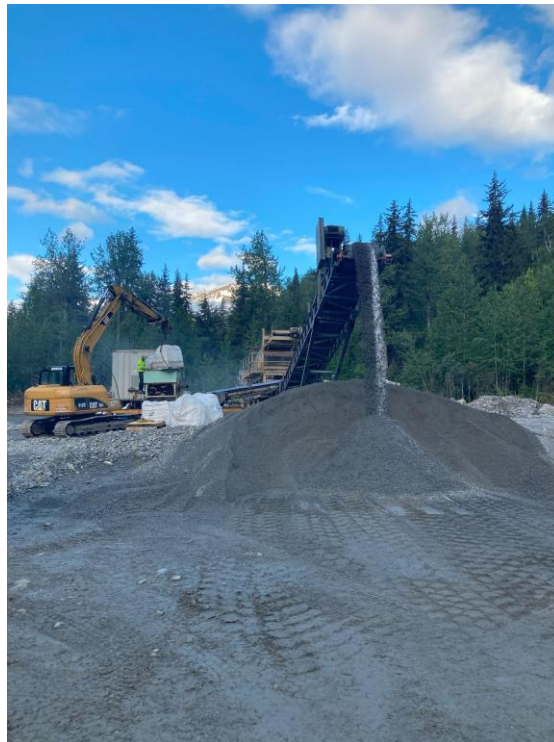
Calcium Chloride and the E material, coming off the belt
