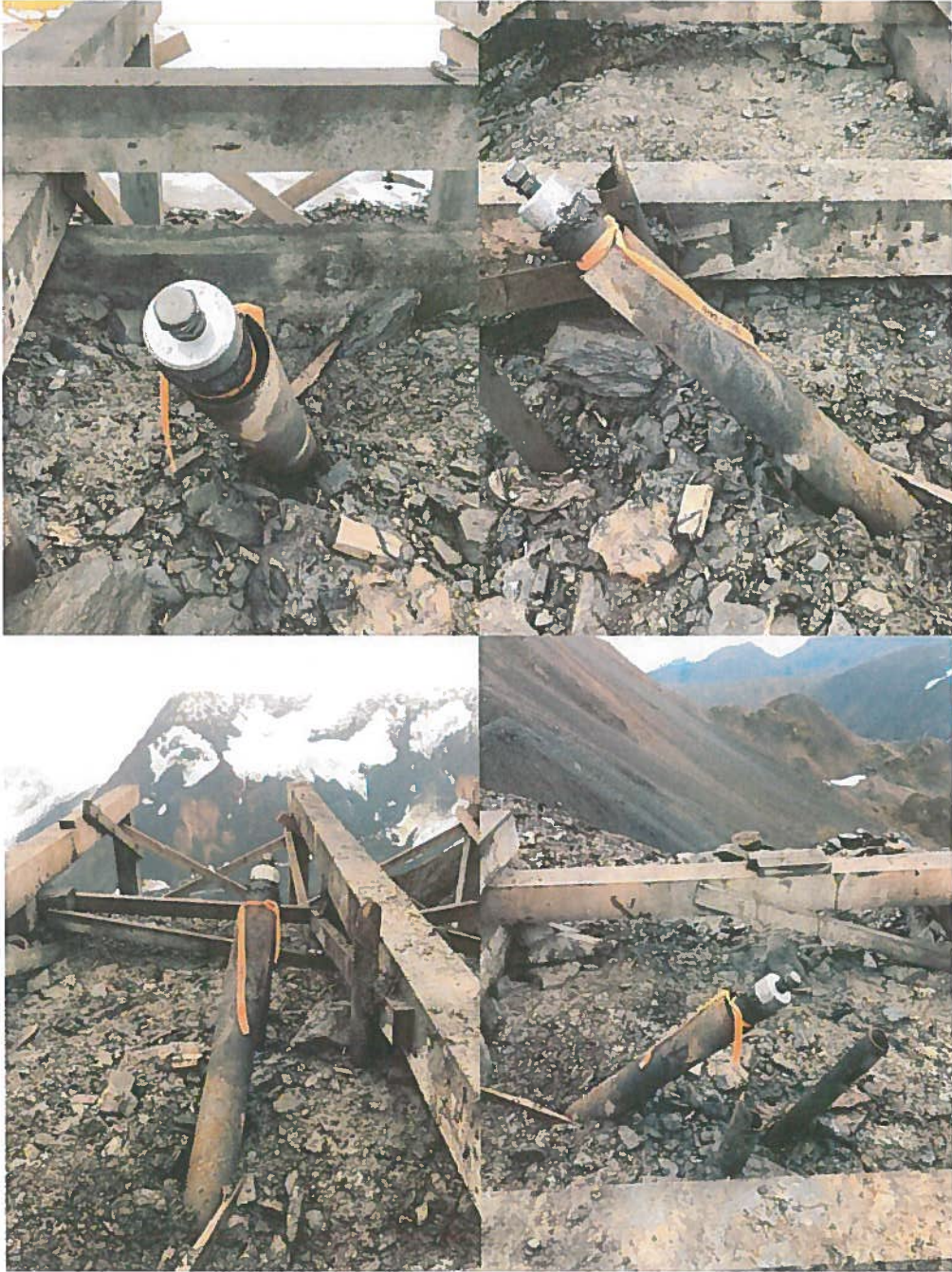
Photo 7: Paradise City Pad diamond drill hole CMR22-148/148B/148C is capped for future re-entrance.
