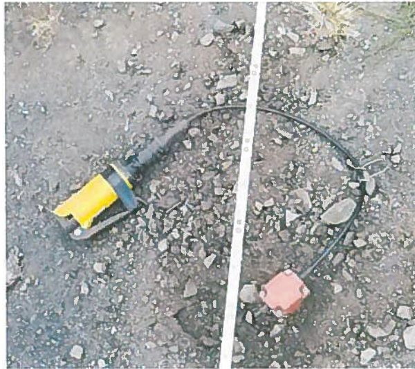
Photo 4 Geophone used for seismic data collection (Palmer Project, 2021)
