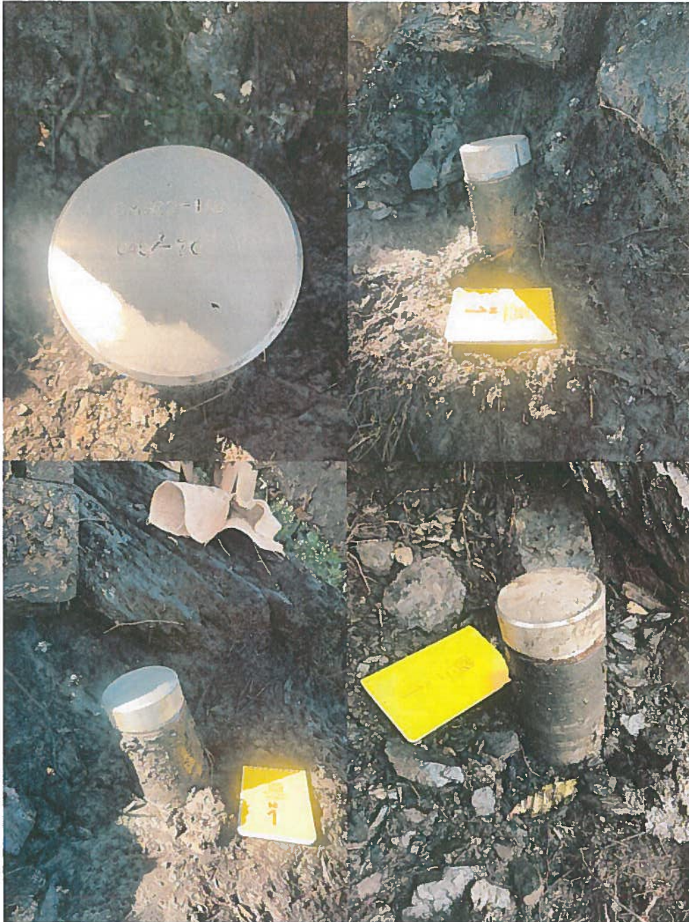
Photo 5: B-Lo Pad diamond drill hole CMR22-146 is capped. Slotted PVC was installed to support potential future tracer studies and geophysical surveys.
