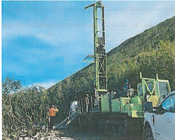
Photo 1 Track Mounted Sonic drill rig (Palmer Project, 2021)
