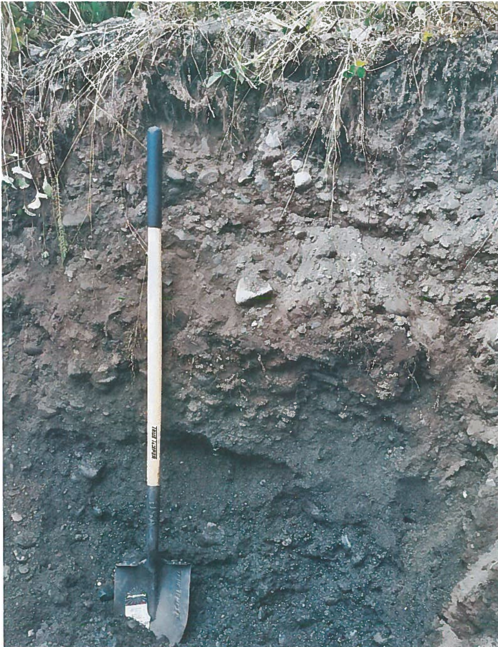
FIGURE 4.2. REPRESENTATIVE HORIZON. TOPSOIL LAYER IS SEVERAL INCHES THICK FOLLOWED BY COARSE GRAINED COBBLY SANDS WITH INTERBEDDED FINER GRAINED BEACH SANDS TYPICAL OF A NEARSHORE MARINE ENVIRONMENT.
