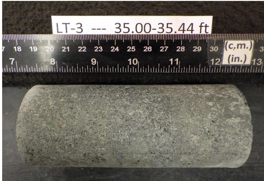
After cutting and grinding
