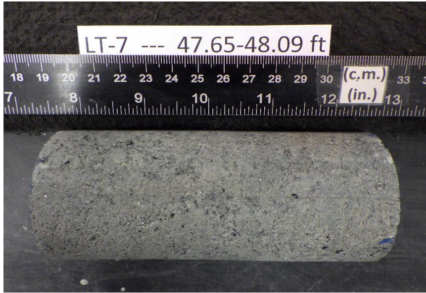
After cutting and grinding
