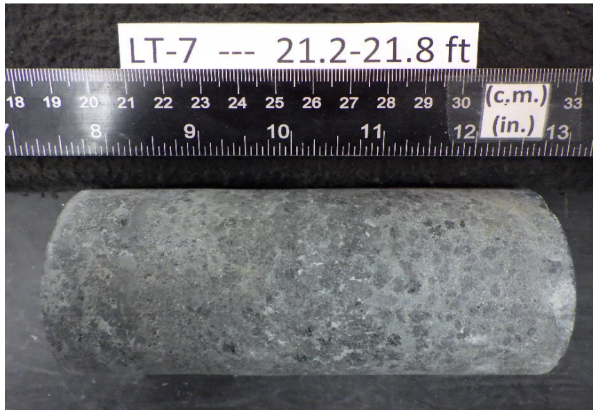
After cutting and grinding
