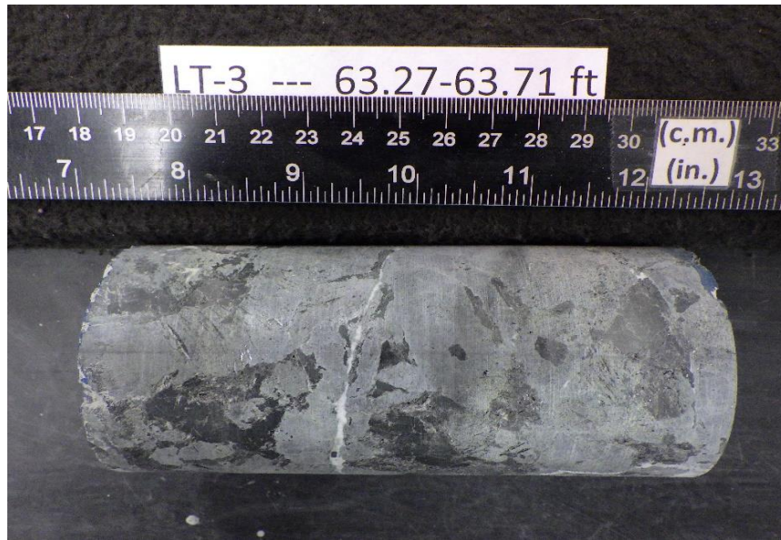
After cutting and grinding
