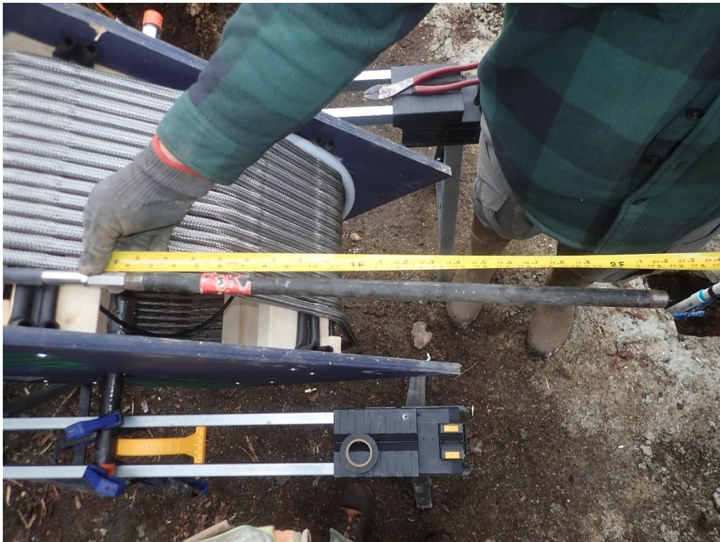
B: Typical 2-foot pipe extension used at LT-1, LT-2, LT-3, and LT-6
