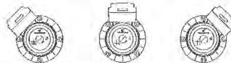
Fig. 1 Possible terminal box positions
