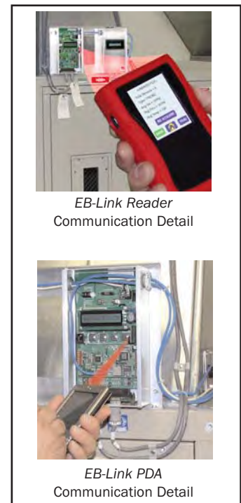
Figure 15. Typical EB-Link Data Acquisition
