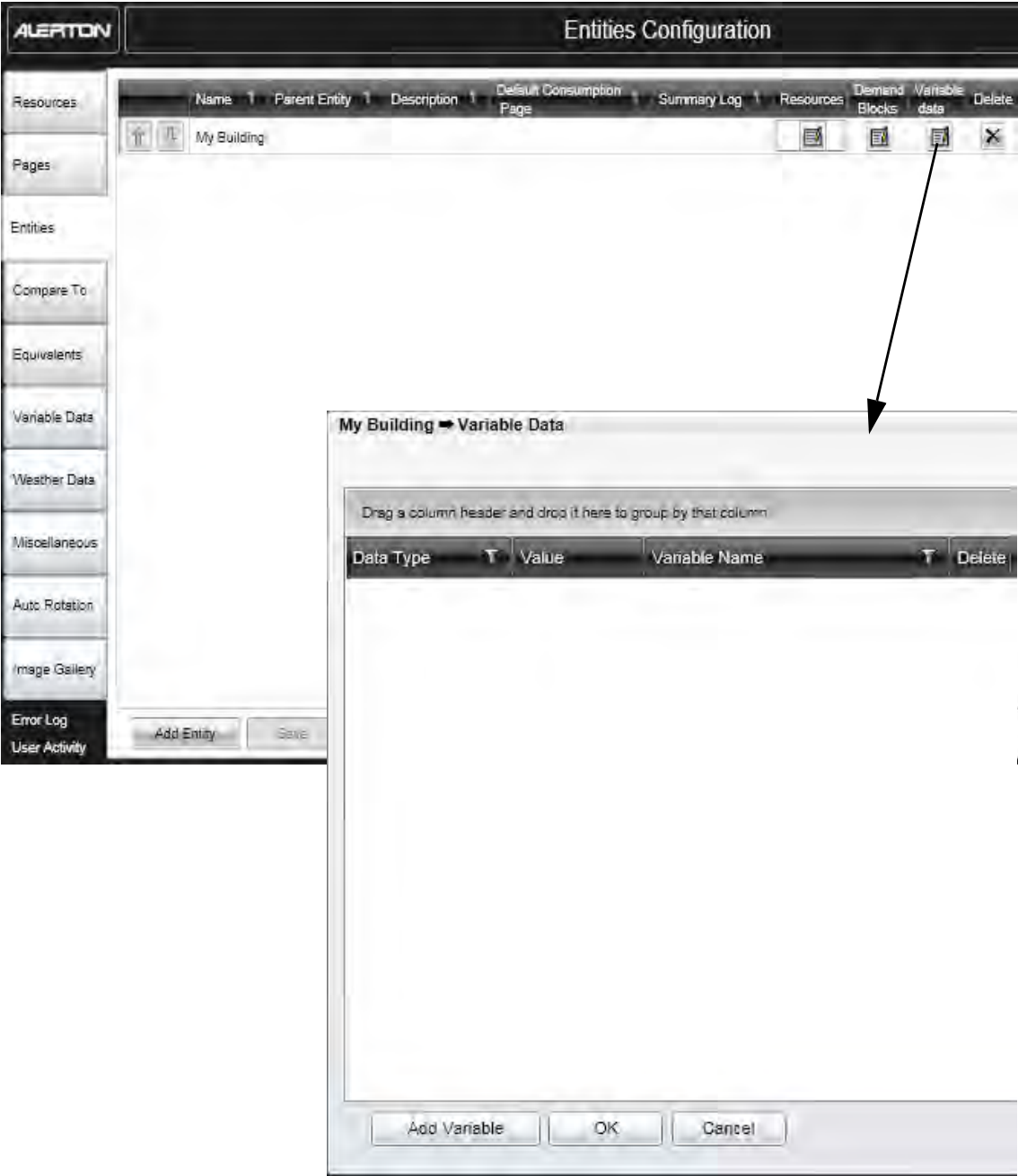
Figure 12.13 Click the Edit Variable Data icon on the Entities page to configure BACnet data to display.
