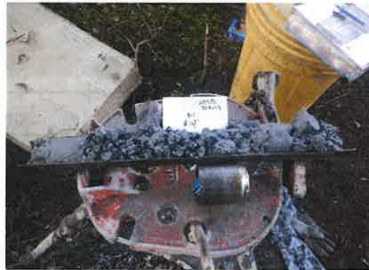
Figure 4-1: Very dense clayey sand with gravel encountered 100 feet bgs in BH-1.
