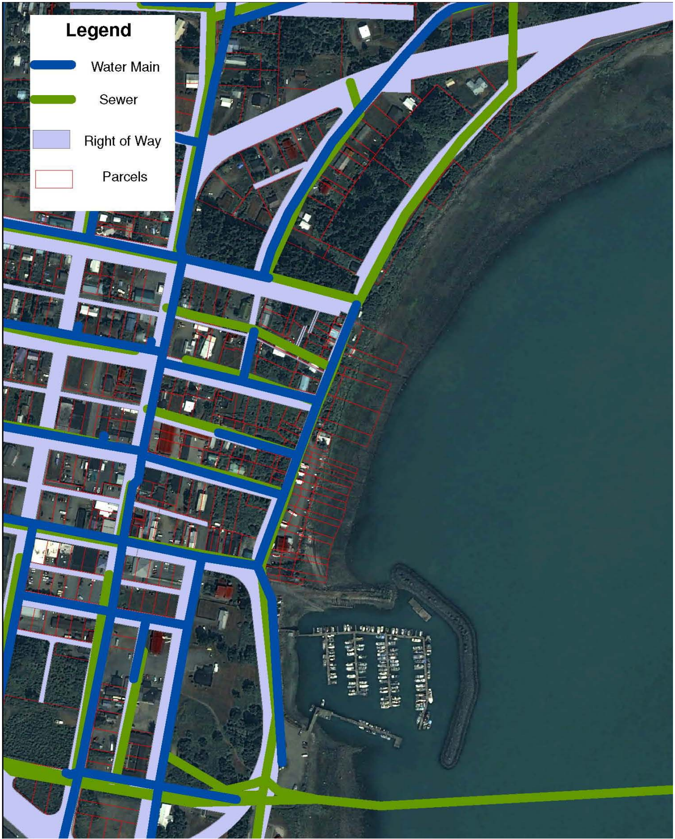
Figure 3-2: Water and Sewer Lines in Vicinity of the Existing Harbor and Proposed Expansion Area.
